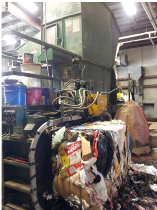
The back of the baler, with a new bale pushed out at the bottom.
