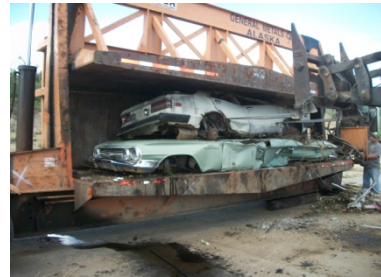
Northern Recycling supplied a car crusher. In efforts by other villages, heavy equipment has been used to crush cars.
