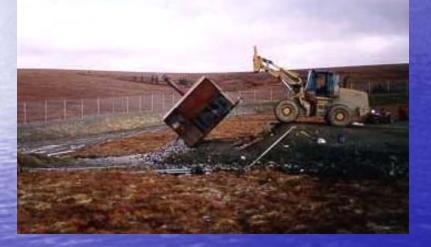
One of the bad things about burning-- You still need to deal with the ash. To empty the ash, people tilt this burnbox with a dozer. But burnboxes can be made with a handle to tilt by hand, or you can shovel the ash out.
