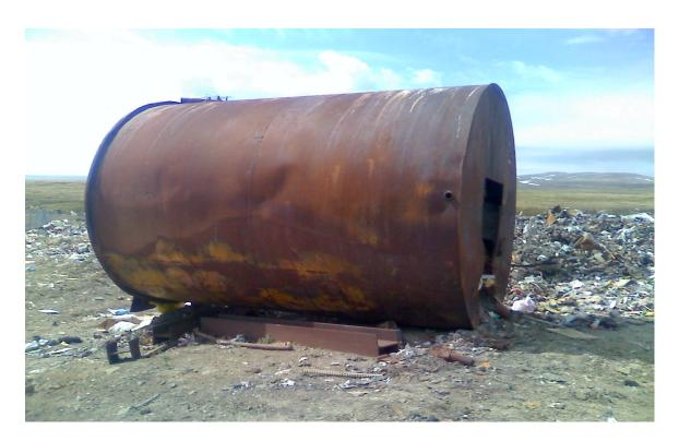
Above is the picture of the burn barrel the refuse workers use to burn materials. It has a small opening at the end of the barrel measuring about 4ft wide x 4ft tall to take out the debris. Too small for any machinery to push back. Need to move debris manually which takes up more time. Manually shovel out and move. With a new burn barrel, it would need to be only tipped so that material can be poured out.
