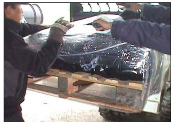
Selawik shrinkwraps and palletizes their batteries to stage them for shipping.
