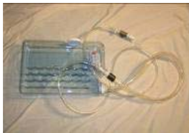
Figure 43: Flexible pvc piping and water container modified for the Envirolet
