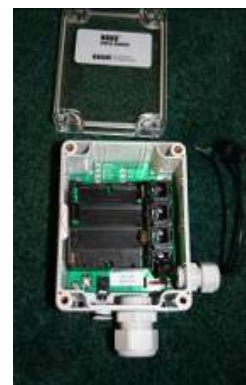
Figure 35: Microstation with four sensor ports
