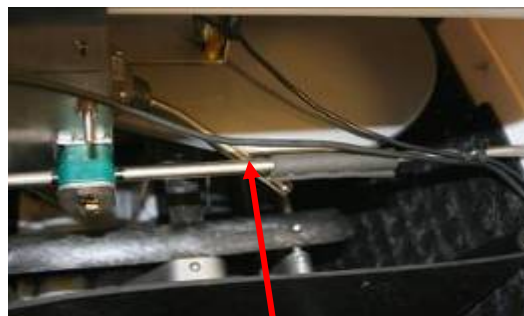
Plastic disk hitting the spring tip switch
