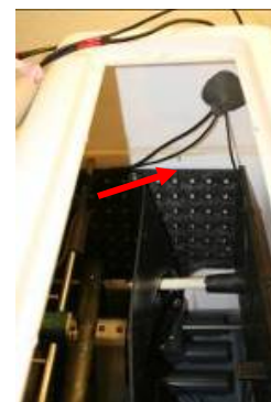
Figure 36: Hole drilled for sensor wires to exit toilet, filled with clay
