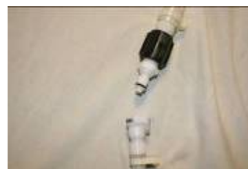
Figure 47: Close-up of the snap valve disconnected
