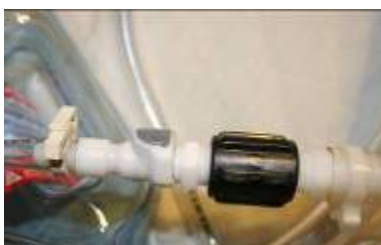
Figure 46: Close-up of the snap valve for leak-free disconnect
