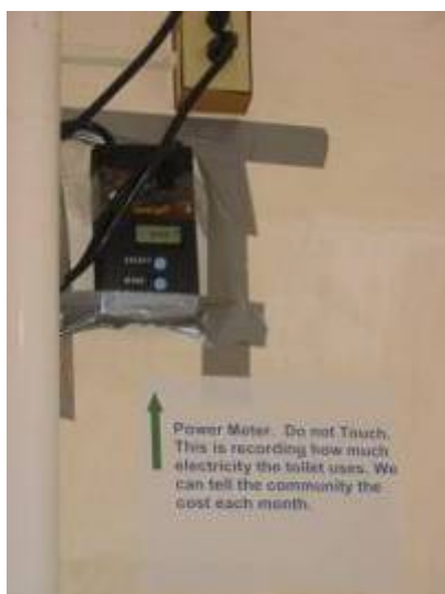
Figure 48: Photo of the Watt's Up meter on the wall above the toilet, with sign for the public
