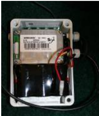
Figure 37: Solar Stream data transceiver box
