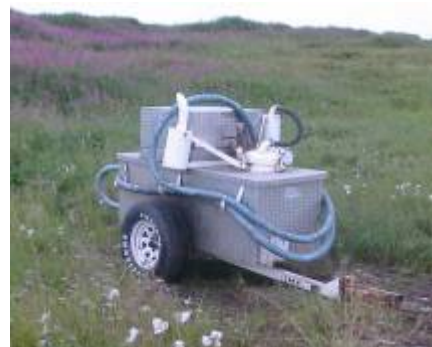
Figure 14: Vacuum tanker used for removing wastewater from flush-haul
